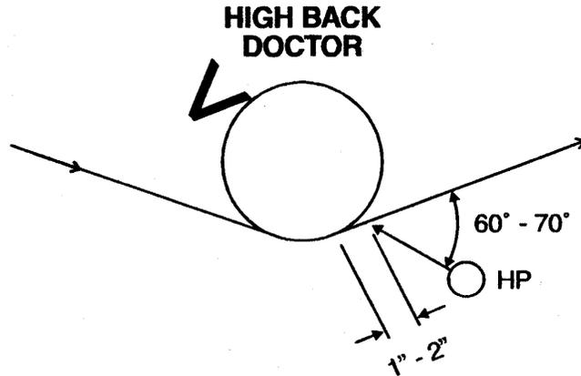
Detail 2: HP shower 60-70 degrees into fabric run, impacting 1"-2" after the fabric leaves the roll.
