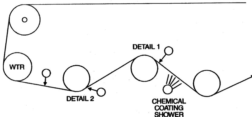
Case 2: If the first return roll is an inside roll, many mills have added an additional outside roll to be able to employ the wash roll doctor sheet knockoff technique. This well proven technique completely eliminates sheet knockoff problems caused by lower CFM multi-layers and CFM reduction with contamination.
