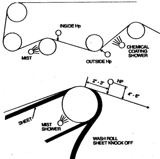
**Detail 1:** HP shower perpendicular to the fabric run, 2"-3" after the fabric leaves the roll.
